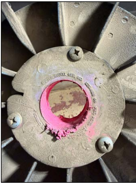
Photos showing melted intake fan from HSI blower motor.
