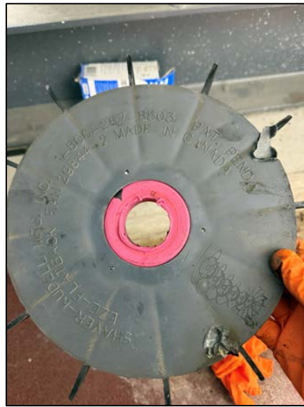
Photos showing melted intake fan from HSI blower motor.
