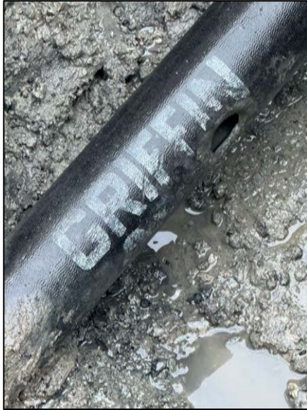
Photos showing the 2" hole and the repair clamp used for the repair.
