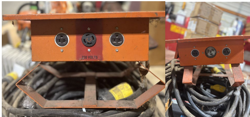
14. 230 volt Distribution Spider Box to power construction sites.
