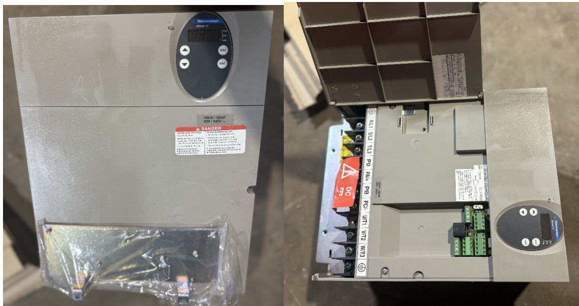
10. 15kW / 20HP – 200 / 240V Telemecanique Altivar 31 Asynchronous Motor controller
