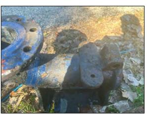
Photo of old base elbow with sheared pegs.
