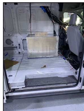
A generator was installed to provide power to the televising camera, cable reel, computer, and control module.
