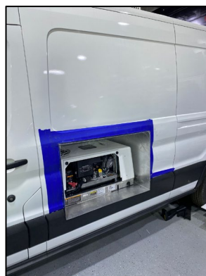
A generator was installed to provide power to the televising camera, cable reel, computer, and control module.
