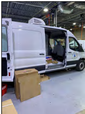
Early stages of televising van upfitting. The HVAC Unit can be seen on the roof, and interior electrical wiring is being installed.
