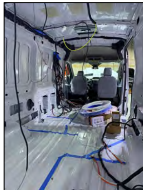
Early stages of televising van upfitting. The HVAC Unit can be seen on the roof, and interior electrical wiring is being installed.
