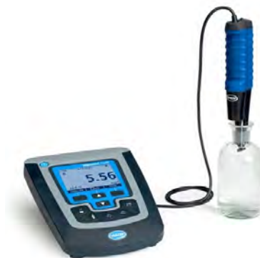
Stock photo of probe inserted in BOD bottle and connected to meter.
