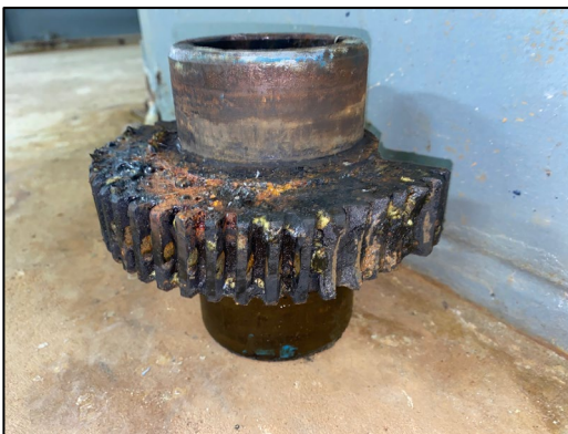
Broken teeth on actuator gear.
