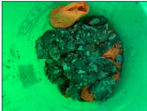
Grease and rags removed from sewer main.
