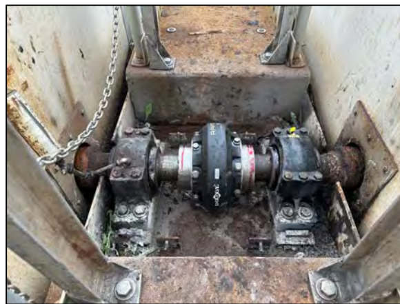
Photo of new Dodge Raptor Coupling after install.
