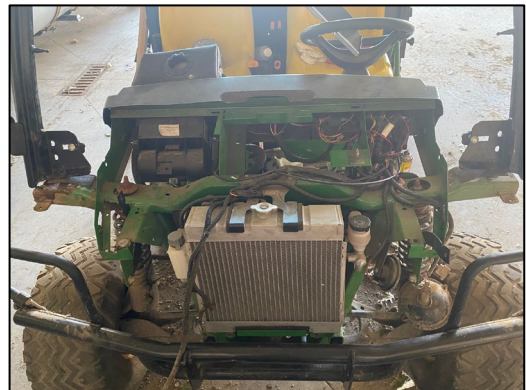
Plastic body has been removed from vehicle chassis.
