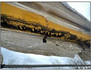
Ruts on underside of old conveyor.
