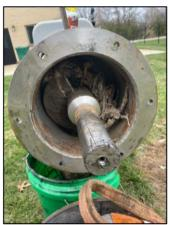
Exposed screw after gearbox removed.
