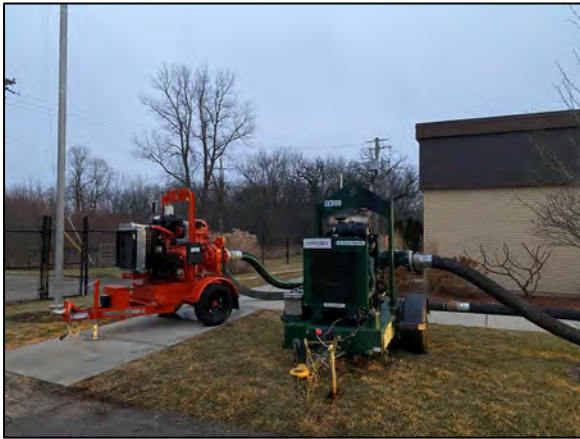
Two bypass pumps used for bypass event.
