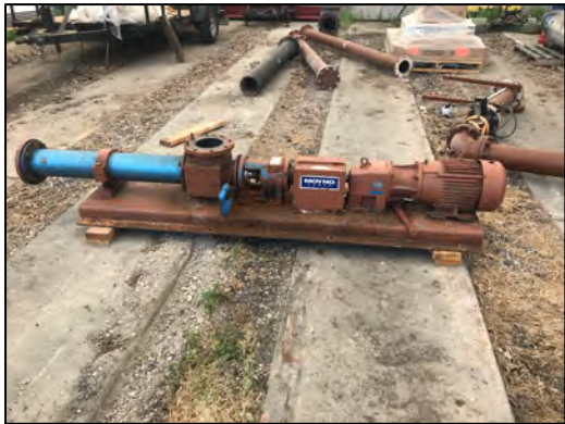
Old Moyno sludge pump after removal.
